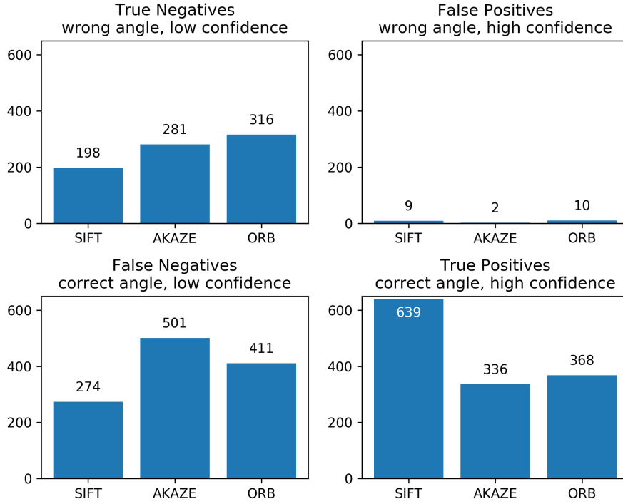
Fig. 4. Confusion matrix of the compass using different algorithms with confidence threshold of 0.5.
