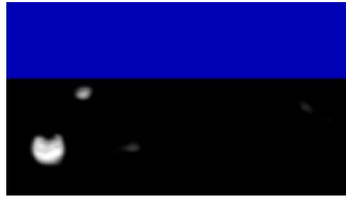
(b) The output of the FCNN based on the input image. The true positive detection of the ball is most prominent in the heatmap while smaller false positive detections of the left goalpost and the penalty mark are visible, too.
